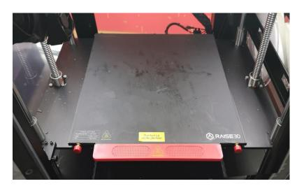
• Tighten the thumb screws to fix the Build Plate. Confirm whether the pate can hardly be moved before shooting a print.
