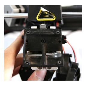
Fix the Protective Cover and Front Fan back onto the Fan Duct with 4 fixing screws.
